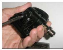
1. Loosen adjusting screw until axle can be moved forward and back easily by hand
