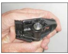
2. Push axle so outer bearing is as far forward as possible
