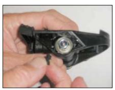
3. Push insert behind bearing with the outer lip sitting over the axle
