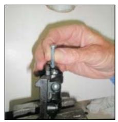
7. Using a suitable drift, lightly tap the insert into place. Replace the end cap. Replace the dust cap.
