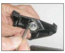
6. Being careful not to damage the axle, place the pedal on its side (in an open vise for example) and position the second insert.
