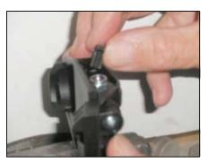
4. Lightly push the insert home with a suitable screwdriver
