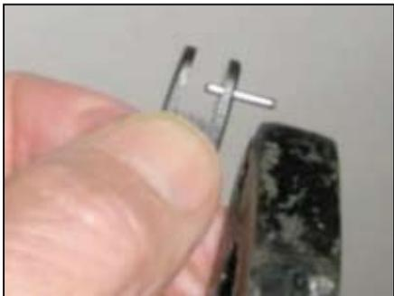
2. Assemble spring on locking pin shaft and insert locking pin in pedal with the chamber facing forward.
