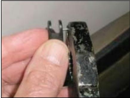
1. Push the roll pin into lever until 3mm exposed on the inner side.
