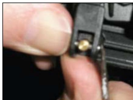
4. Use grips as shown to push home the roll pin. Use a screwdriver blade to adjust the pin to be positioned symmetrically and ensure the lever works smoothly.
