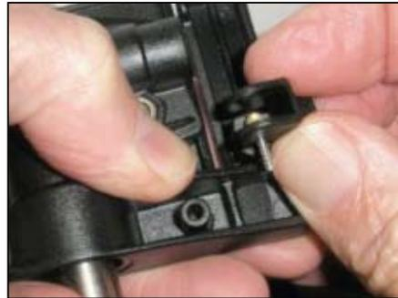
3. Hold the pedal in one hand with the locking pin pushed into the pedal. Slide lever/roll pin assembly over the end of the pin and insert the roll pin into the hole in the locking pin.
