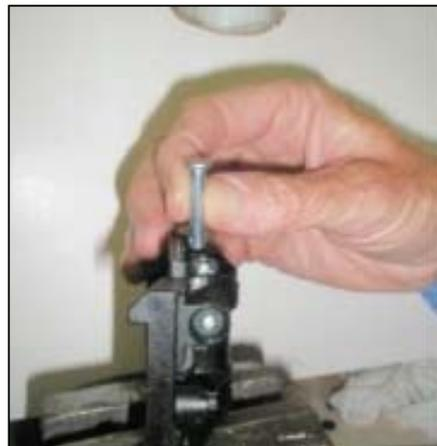
7. Using a suitable drift, lightly tap the insert into place. Replace the end cap. Replace the dust cap.
