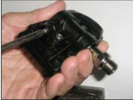
1. Loosen adjusting screw until axle can be moved forward and back easily by hand
