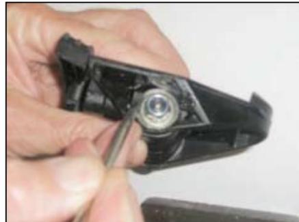
6. Being careful not to damage the axle, place the pedal on its side (in an open vise for example) and position the second insert.
