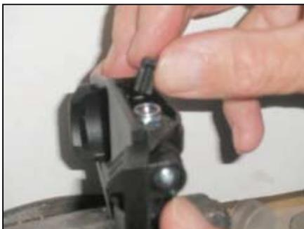
4. Lightly push the insert home with a suitable screwdriver
