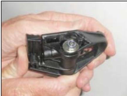
2. Push axle so outer bearing is as far forward as possible
