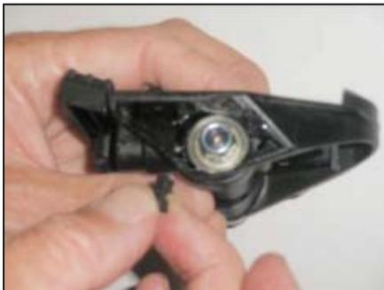
3. Push insert behind bearing with the outer lip sitting over the axle
